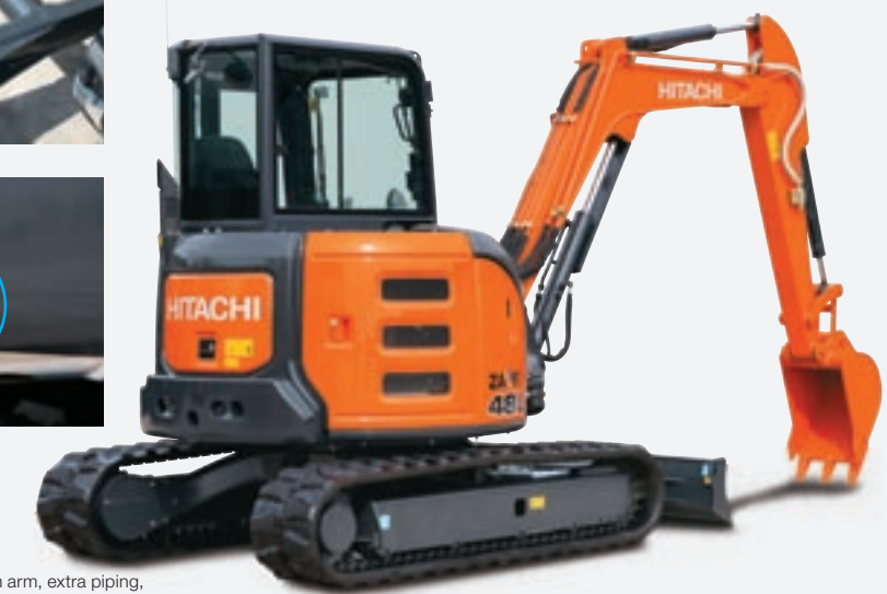
Shown equipped with 1.69 m arm, extra piping, additional counterweight, rear view mirror and stack muffler.
